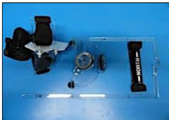
Figure 1: Back range of motion (BROM) device: It consists of two plastic units: an inclinometer for measuring pelvic inclination and sagittal plane motion and a combination gravity goniometer/compass for side bending and rotational motions respectively
